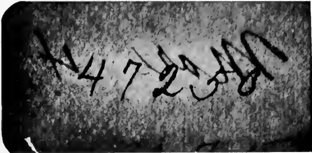
FIG. 6—Transmitted light photograph, showing erasure by abrasion. "Mar. 4" on opposite side of sheet.
